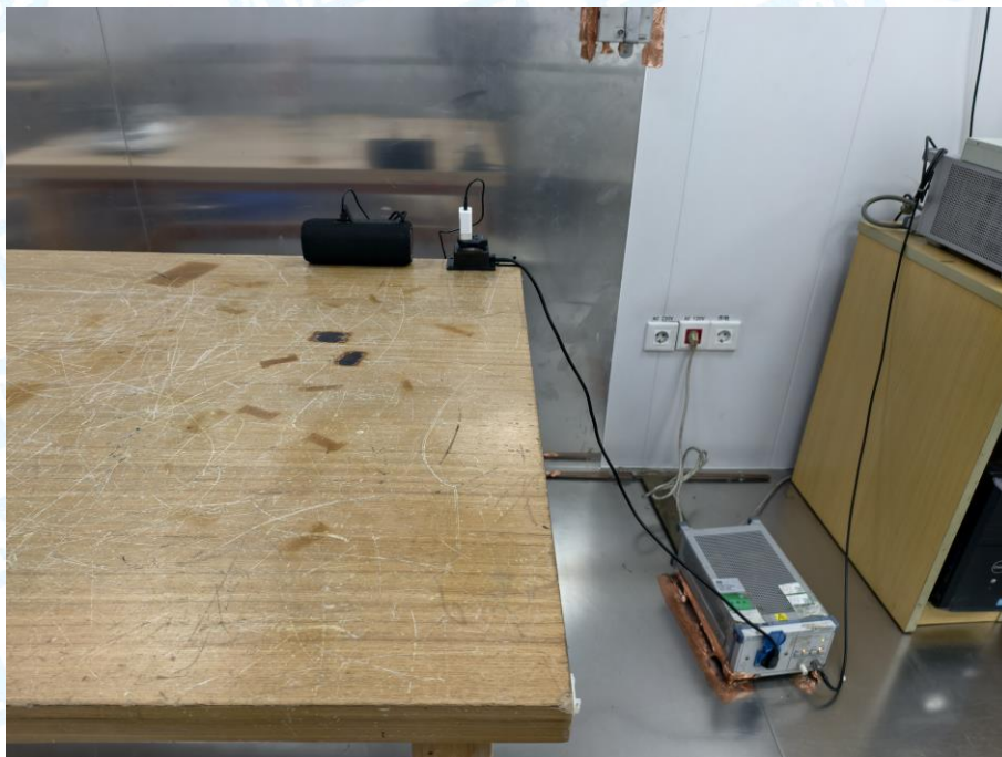
Photo of Setup for Conducted Emission
