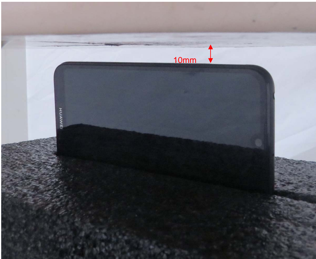
Picture 10: Left Side, the distance from handset to the bottom of the Phantom is 10mm
