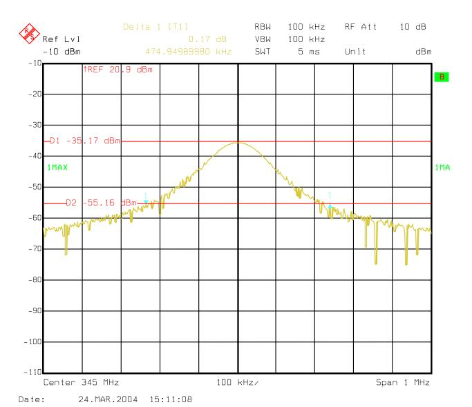
EXHIBIT5.4: CFS8DL5809EN-1 OCCUPIED BANDWIDTH (474.95KHz)
