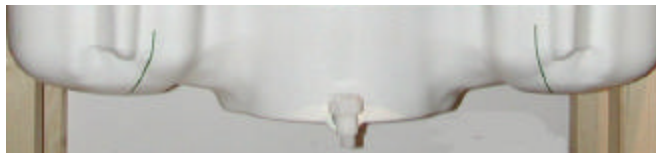
Figure 8.2 SAM Twin Phantom shell
