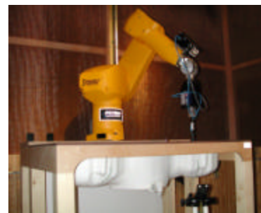
Figure 7.1 DASY3 Test System
