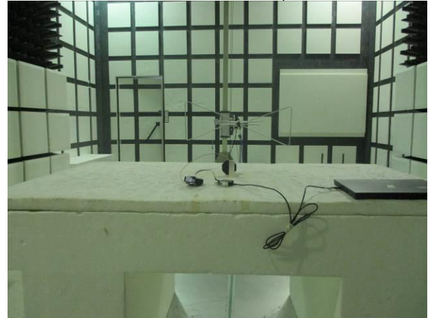
FCC_15_247+IC_RSS_247_902~928MHz_FSK_Radiated_ External antenna_Setup
