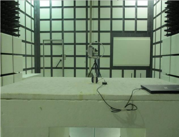
FCC_15_247+IC_RSS_247_902~928MHz_FSK_Radiated_ External antenna_Setup
