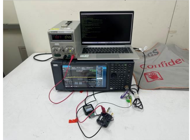
FCC_15_247+IC_RSS_247_902~928MHz_FSK_Radiated_ Internal antenna_Setup
