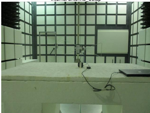
FCC_15_247+IC_RSS_247_902~928MHz_LoRa_Radiated_ Internal antenna_Setup
