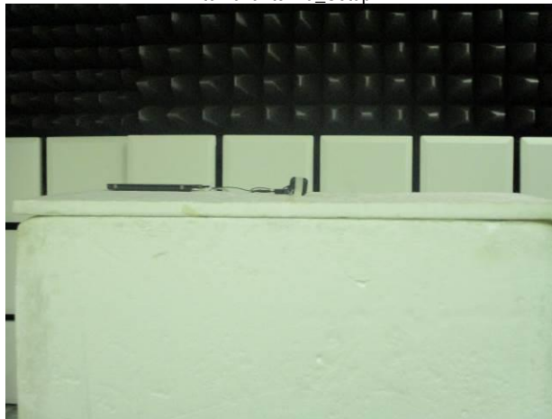
FCC_15_247+IC_RSS_247_902~928MHz_LoRa_Radiated_ Internal antenna_Setup
