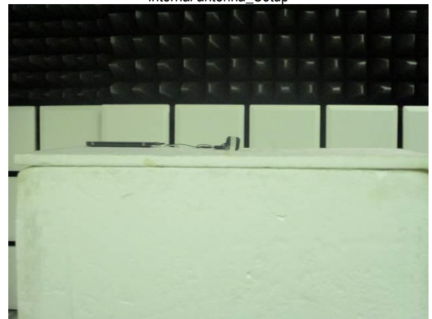
FCC_15_247+IC_RSS_247_902~928MHz_FSK_Radiated_ Internal antenna_Setup
