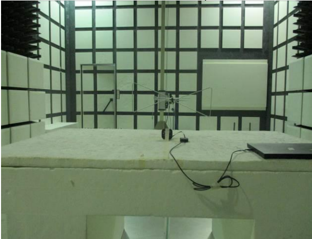
FCC_15_247+IC_RSS_247_902~928MHz_FSK_Radiated_ Internal antenna_Setup
