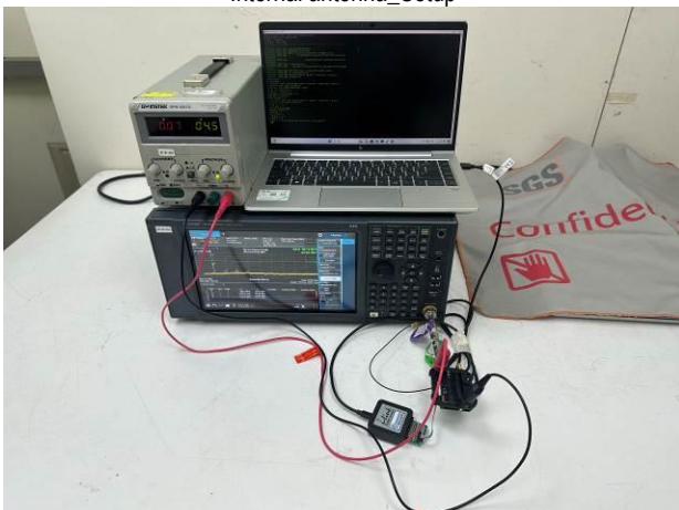
FCC_15_247+IC_RSS_247_902~928MHz_LoRa_Conducted_ Internal antenna_Setup
