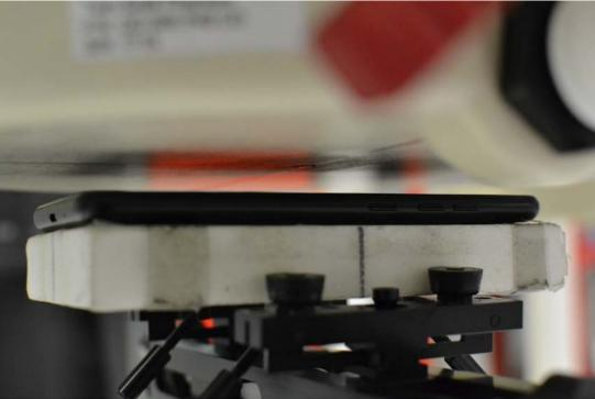
SAR Test Setup Photo 6 – Front at 10mm
