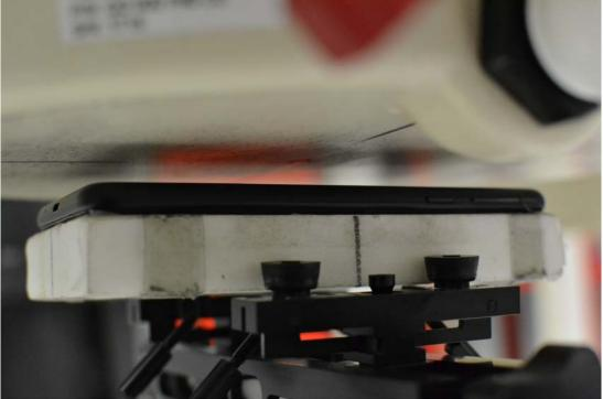
SAR Test Setup Photo 5 – Back at 10mm
