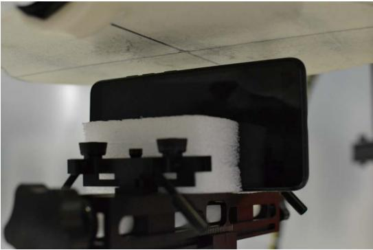
SAR Test Setup Photo 9 – Right at 10mm
