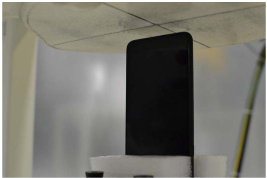
SAR Test Setup Photo 8 – Bottom at 10mm
