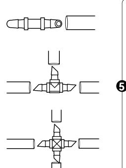
Connecting the suitable barb fitting: 1) If only the hose needs to be connected, **you can use straight barb fitting.**
