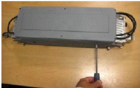
Figure 18 – Attaching front mount antenna assembly to AirSynergy
