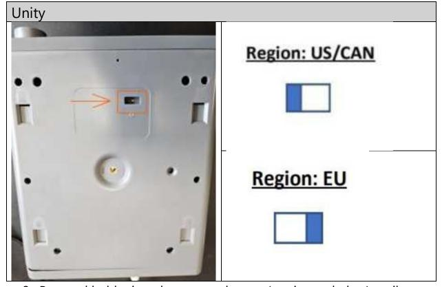
3. Pres and hold microphone mute button (see image below) until microphone beeps **two** times, then release. On Unity, press microphone button once. Then both wireless and battery LEDs on
