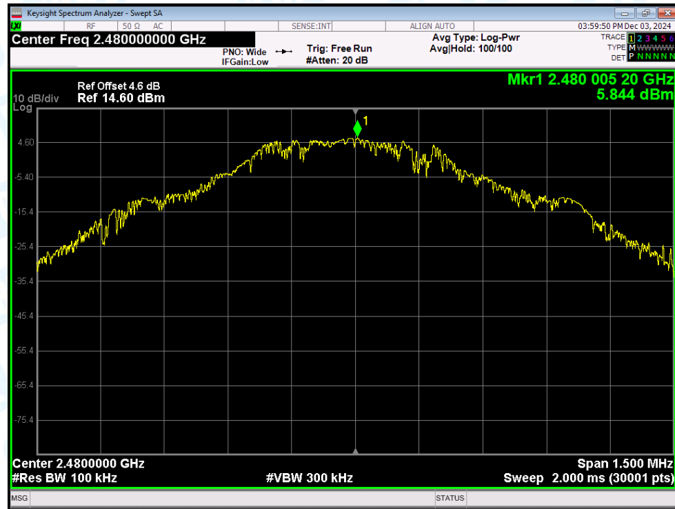
Tx. Spurious NVNT 1-DH1 2480MHz Ant1 Emission
