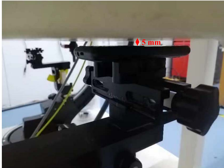
Body (Worn) Front Setup Photo (5mm)
