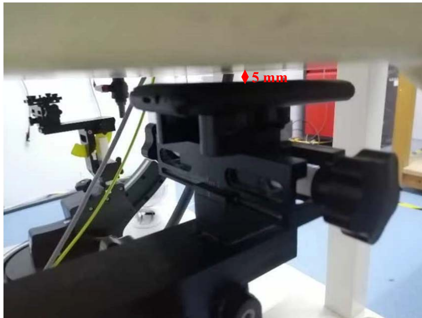
Body (Worn) Back Setup Photo (5mm)
