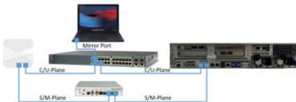
Figure 36 O-RU O-DU connectivity with Switch and GM
