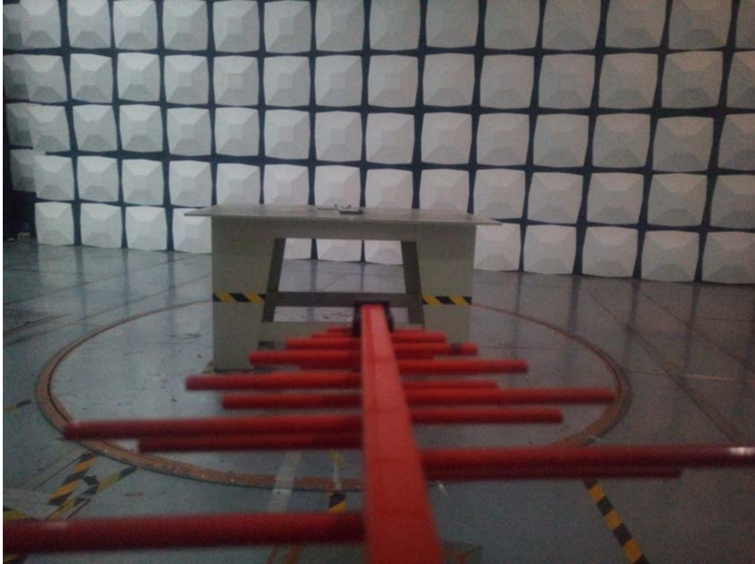
Radiated Emission Above 1GHz front View
