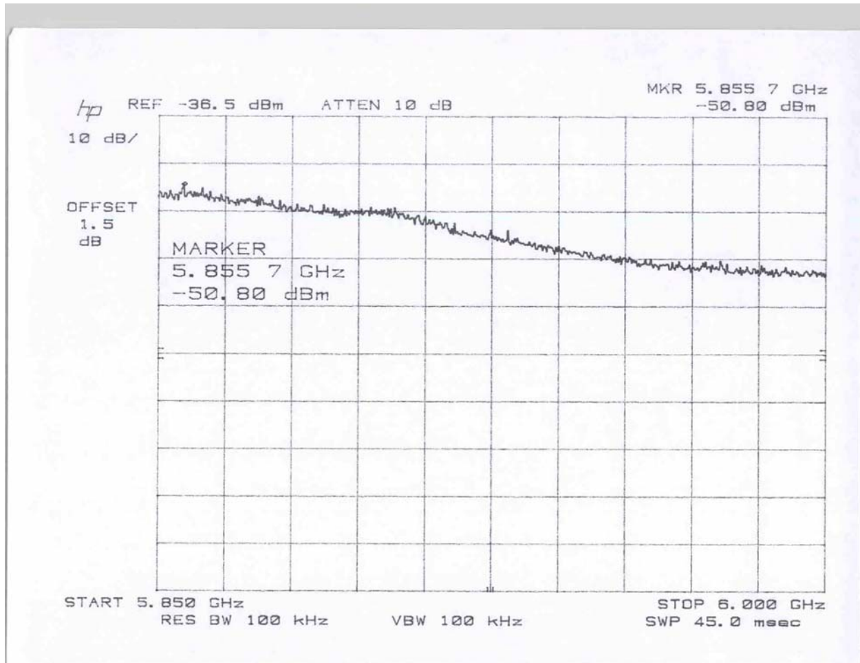
Plot 4.5b High Channel with QPSK \frac{3}{4} modulation and an antenna connector
