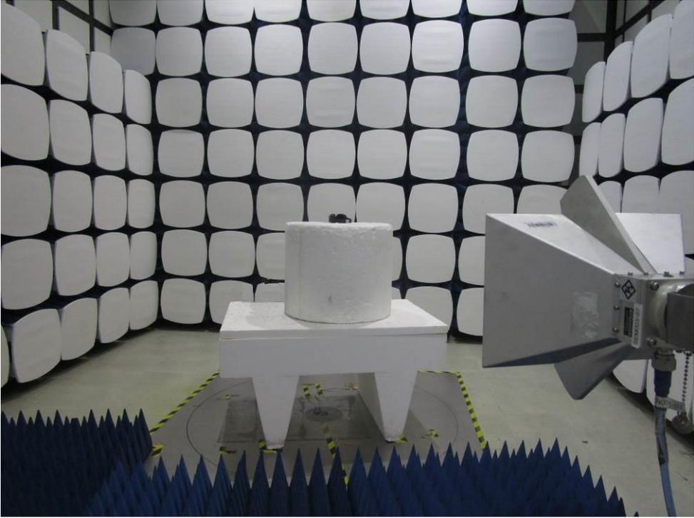
**1.2 Radiated Spurious Emissions Test Setup**
