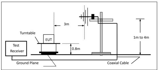
(c) For radiated emissions above 1000MHz
