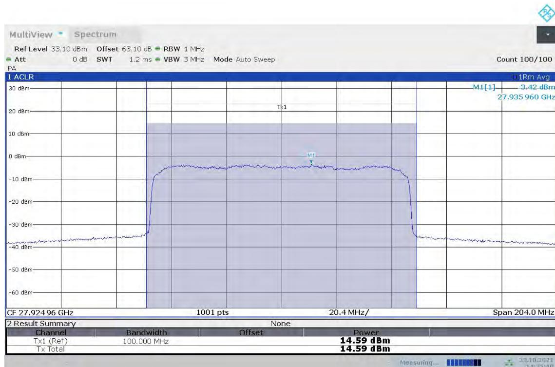
**n261, Module0, 100MHz Bandwidth, 100% RB, MID CHANNEL, 64QAM**
