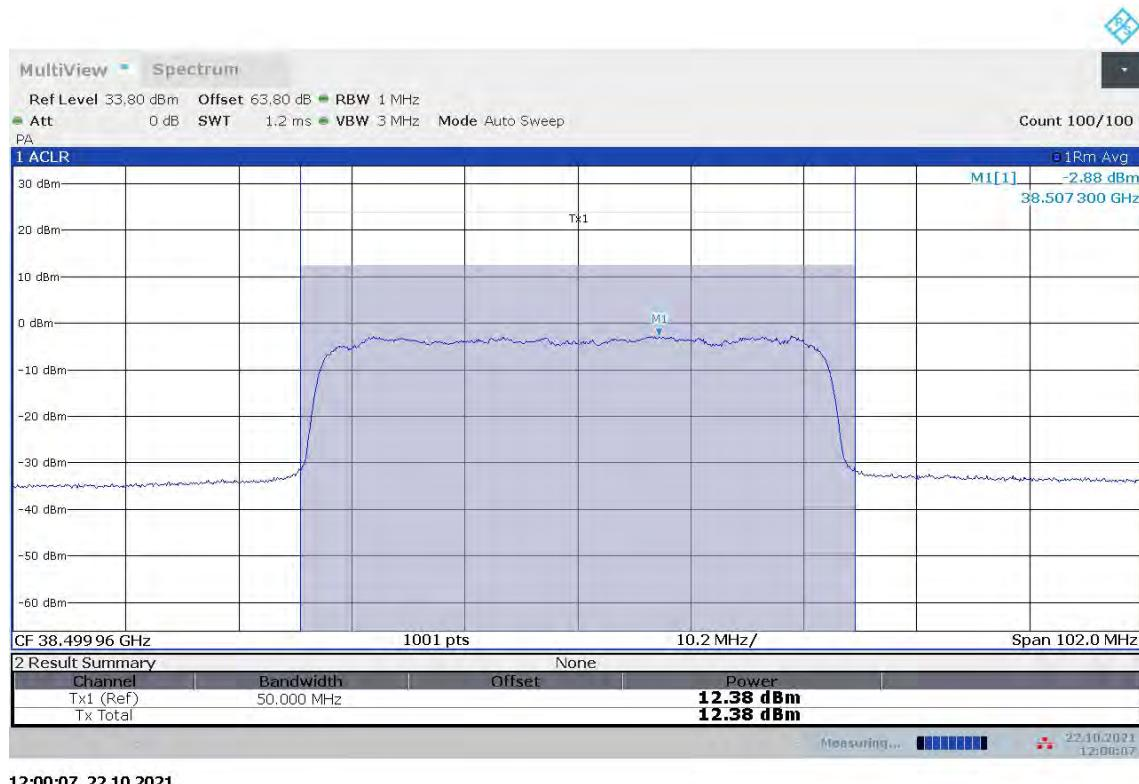
**n260, Module0, 50MHz Bandwidth, 100% RB, MID CHANNEL, 16QAM**
