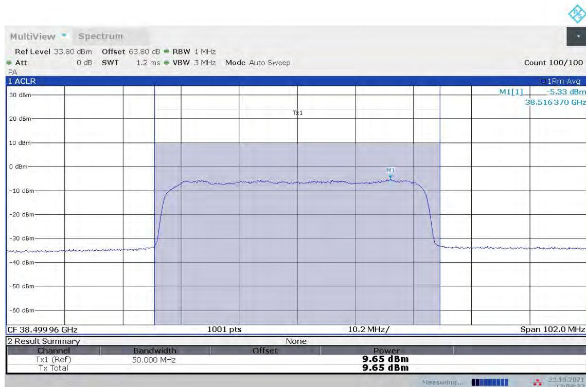
**n260, Module0, 50MHz Bandwidth, 100% RB, MID CHANNEL, 64QAM**
