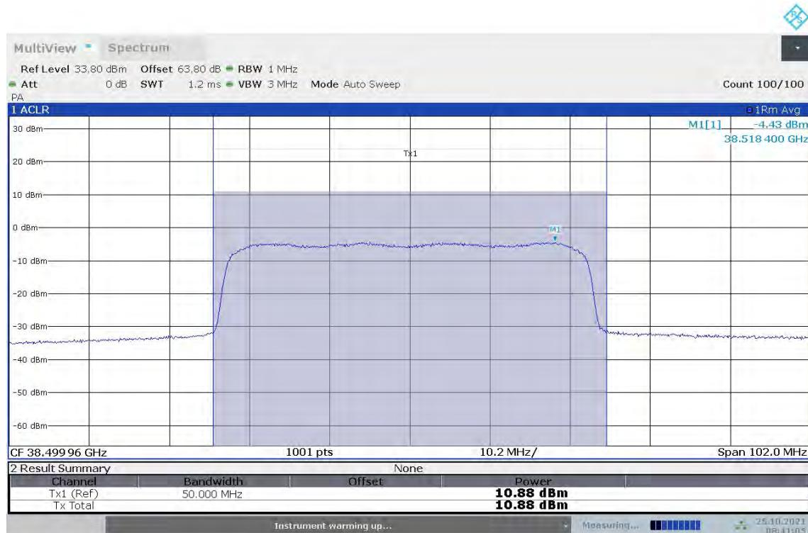
**n260, Module0, 50MHz Bandwidth, 100% RB, MID CHANNEL, 16QAM**
