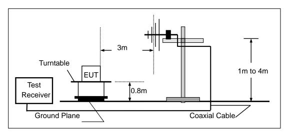
(c) For radiated emissions above 1000MHz
