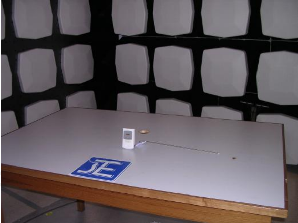
Measurement of Radiated Emission Test Set Up
