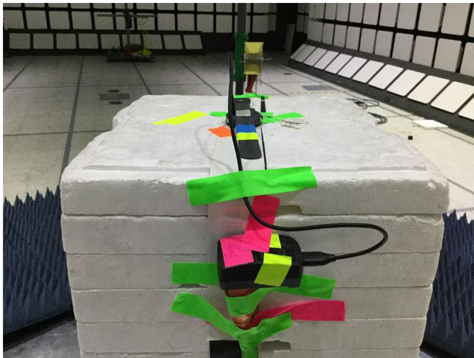
1 – 26 GHz Test Setup
