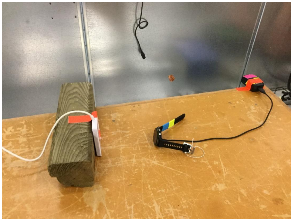
Conducted emissions test setup, NFC
