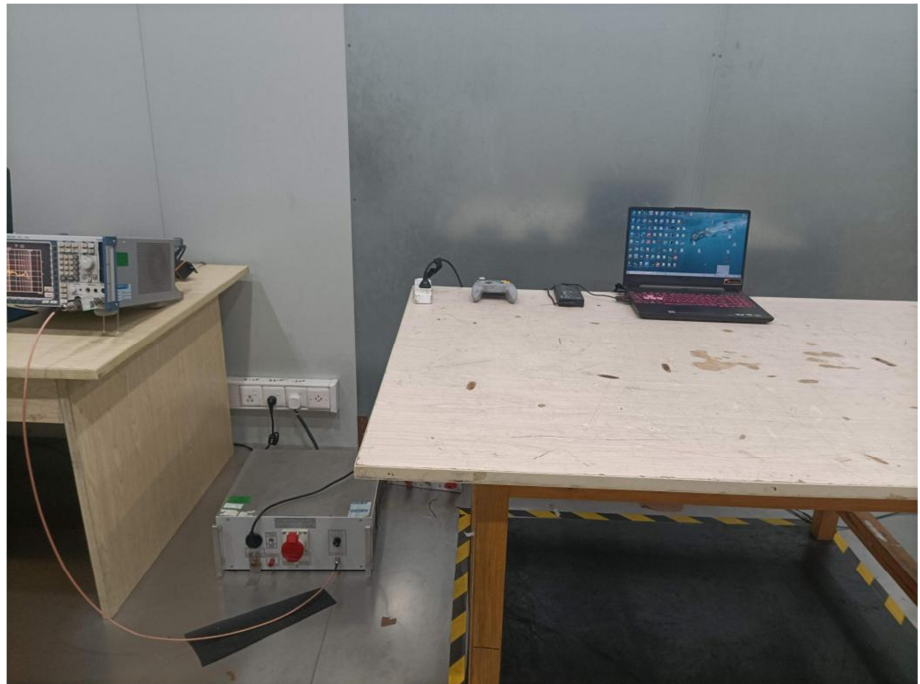
Conducted Emission Test Setup
