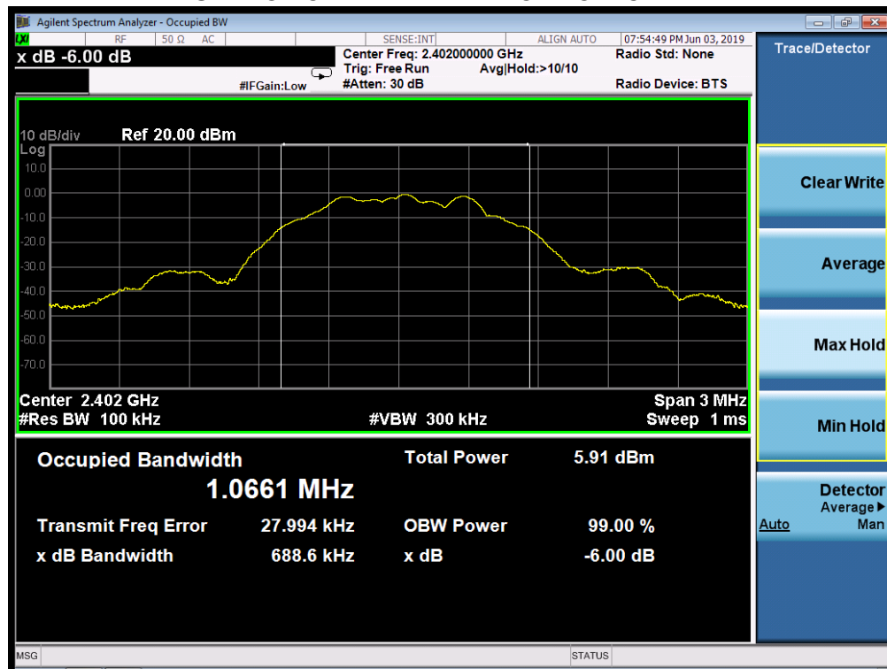
TEST PLOT OF BANDWIDTH FOR LOW CHANNEL
