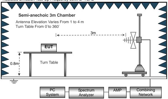
(C) Radiated Emission Test-Up Frequency Above 1GHz
