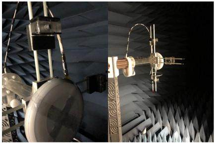
3. Measure the 3D passive performance according to the following coordinate axis.
