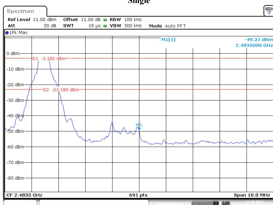
**EDR ( $\pi/4$ -DQPSK): Band Edge-Left Side Hopping**
