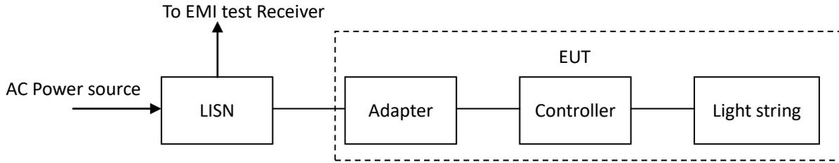
Note: for detail, please refer to the test setup photo for each test item
