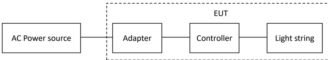
Note: for detail, please refer to the test setup photo for each test item
