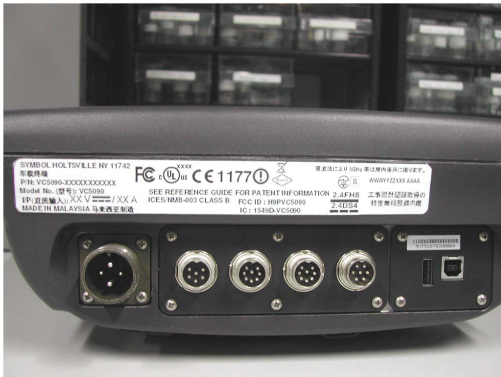
Physical Location of FCC Label on EUT
