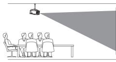
2 To adjust projection to the correct position, press ♠, and select Settings - Advanced Settings - Projection Location - Front Ceiling.
