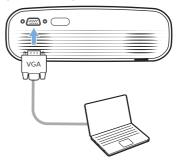
2 On your computer, adjust the screen resolution of the computer to the correct setting and switch the VGA signal to an external monitor. The following resolutions are supported:
