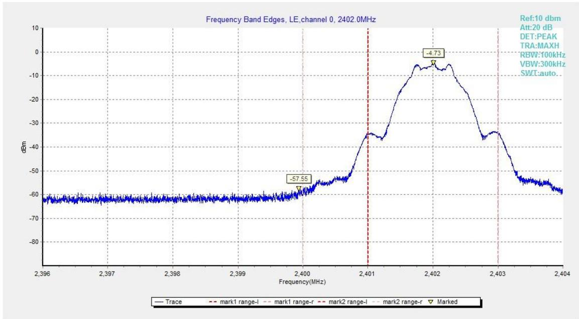
Fig.1. Frequency Band Edges: GFSK, 2402 MHz, Hopping Off
