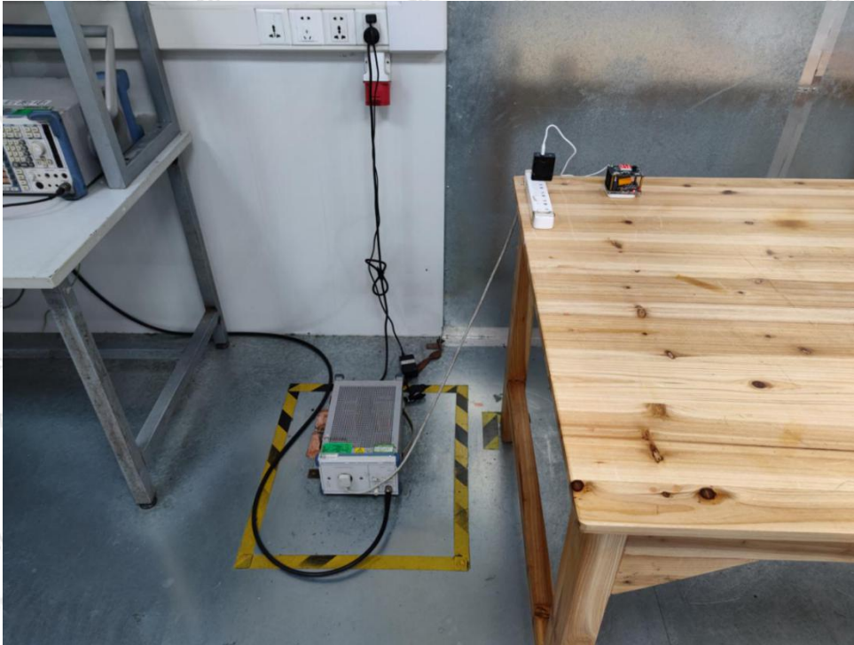
Photo of Conducted Emission Measurement
