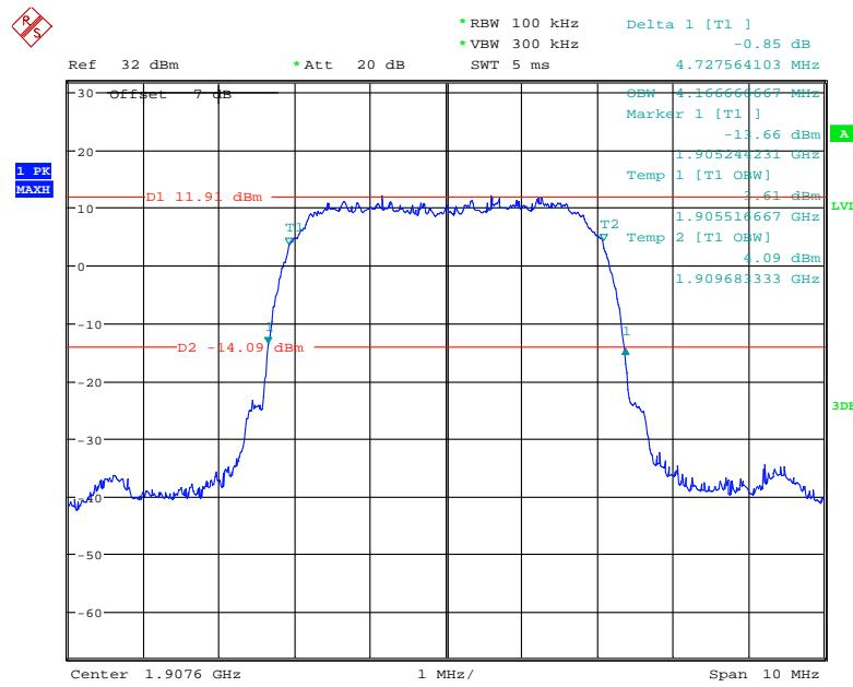
**AWS Band (Part 27)****26 dB Emissions &99% Occupied Bandwidth for RMC (BPSK) Mode, Low channel**
