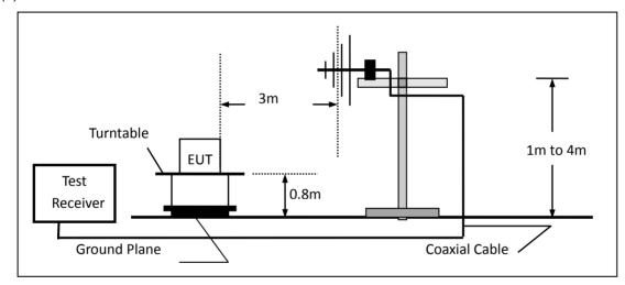
(c) For radiated emissions above 1000MHz
