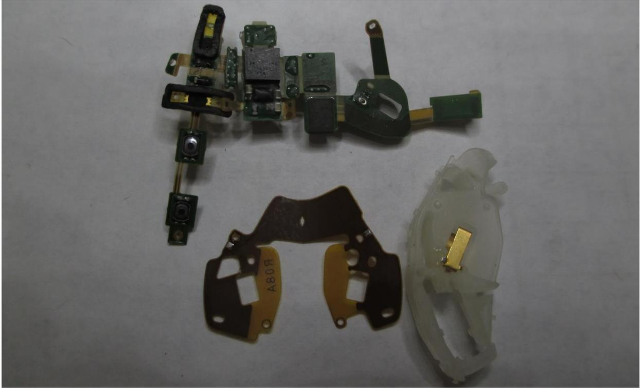
Unfolded flex circuit and 2.4 GHz antenna, bottom view
