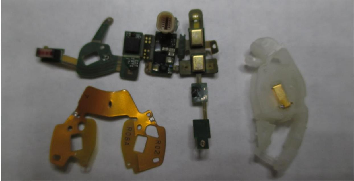
Unfolded flex circuit and 2.4 GHz antenna, top view
