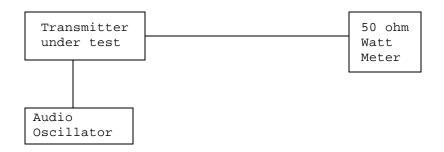
POWER OUTPUT: The RF power output was measured at the antenna feed point using a power meter.
