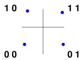
Therefore for the BIT sequence 0 0 1 1 1 0 0 1 The corresponding phase shift will be used
