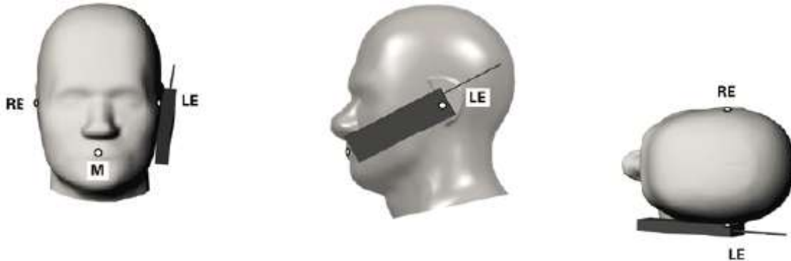
Fig. 11.3 Illustration for Cheek Position
