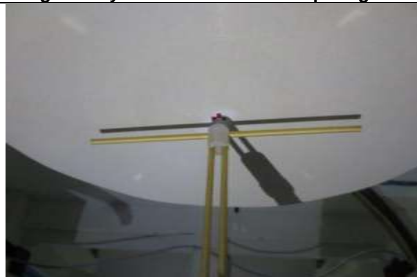
Fig.10.2 Photo of Dipole setup
