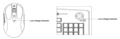
Note: The LED on Mouse can't light when the batteries no power.
