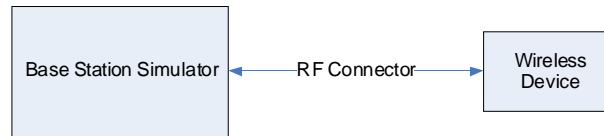
Figure 9-3 Power Measurement Setup
