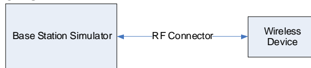
Figure 9-2 Power Measurement Setup
