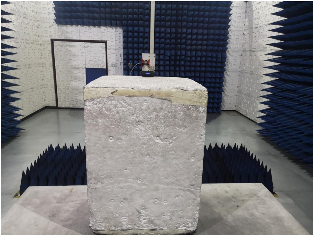
RADIATED EMISSION TEST SETUP ABOVE 1GHz
