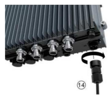
9. Connect and screw the ground cable at the M2RU's left side.
