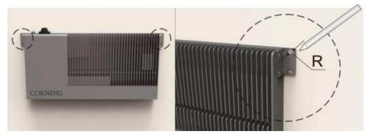
2. Mark 4 x Ø6.8 mm drilling holes sites for the hanger to be attached to the wall.
