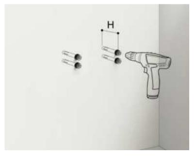
5. Attach the dowels, expansion screws or the like and fasten the Bracket II to the wall.
