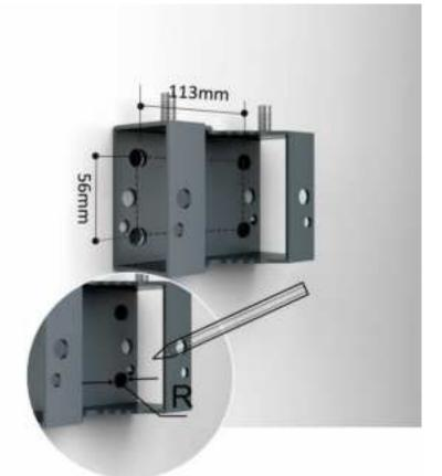
4. Drill 4 holes at the marked positions. Note: H = 70 mm.
