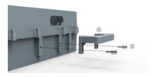
2. Attach and fasten the Bracket I to the back of M2RU with screws M6×14 using T5 Wrench.
