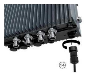
9. Connect and screw the ground cable at the M2RU left side.
