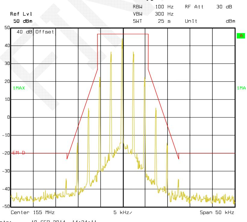
**Occupied Bandwidth – FM, 155 MHz, Low Power Level**
