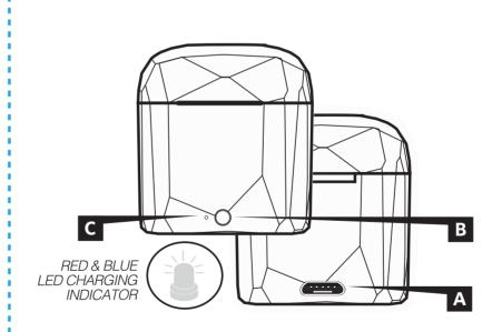
A MICRO-USB CHARGING PORT B POWER BUTTON C LED INDICATOR
