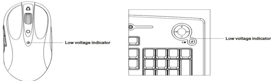
**Note: The LED on Mouse can't light when the batteries no power.**
