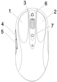
1. There are two additional 4 and 5 on left side on mouse. The two buttons are using in page-up and page-down on acquiescence operating system. You can set-up this two button as you like when installing CD driver.
