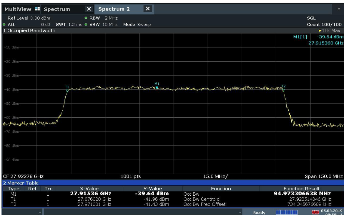
Plot 7-7. Occupied Bandwidth Plot (1CC-100MHz Bandwidth QPSK Mid Channel)
