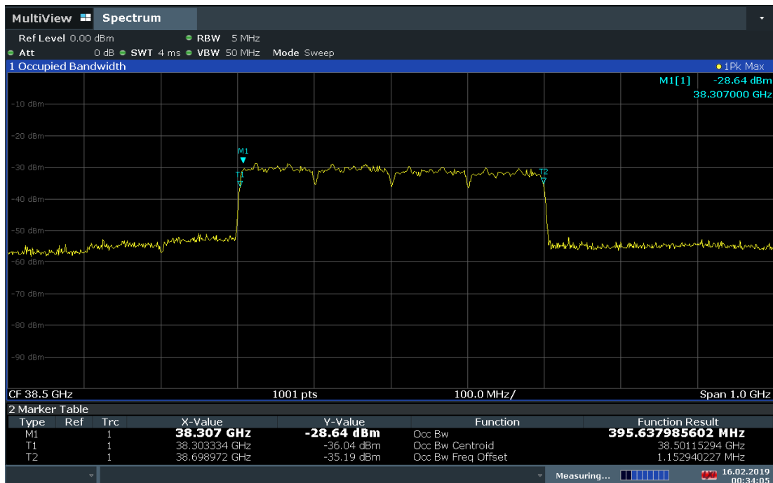
Plot 7-48. Occupied Bandwidth Plot (4CC-100MHz Bandwidth 64QAM Mid Channel)
