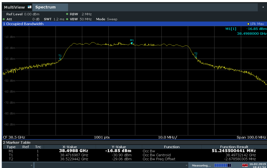
Plot 7-39. Occupied Bandwidth Plot (1CC-50MHz Bandwidth 64QAM Mid Channel)
