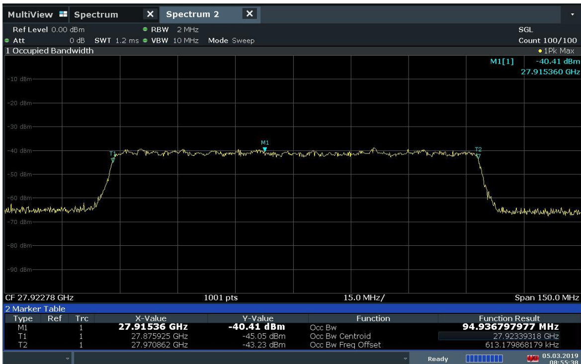
Plot 7-33. Occupied Bandwidth Plot (1CC-100MHz Bandwidth 64QAM Mid Channel)
