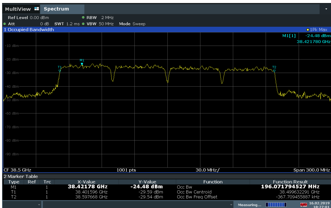
Plot 7-17. Occupied Bandwidth Plot (4CC-50MHz Bandwidth 16QAM Mid Channel)
