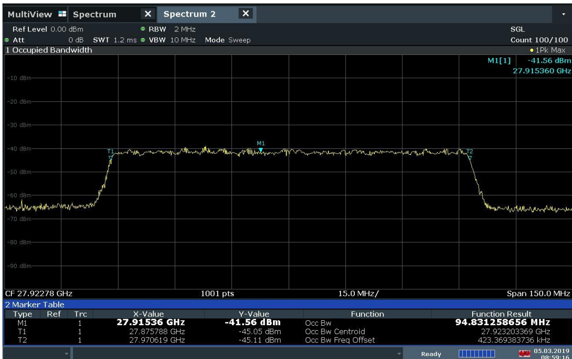
Plot 7-9. Occupied Bandwidth Plot (1CC-100MHz Bandwidth 64QAM Mid Channel)
