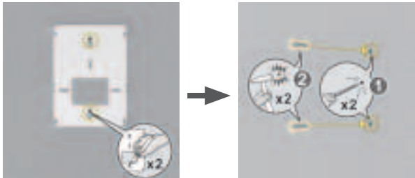
FIGURE 9>10: Mark the positions of the two screw holes and make the screw holes.
