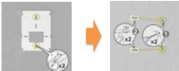
FIGURE 9 Mark the positions of the two screw holes and make the screw holes
