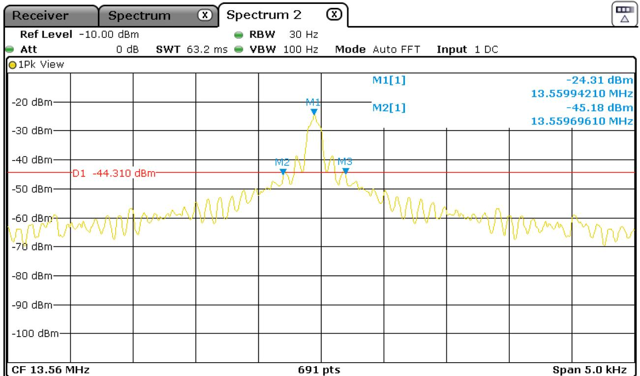
Figure 14: Chart of 20 dB bandwidth tests, without tag, USB
