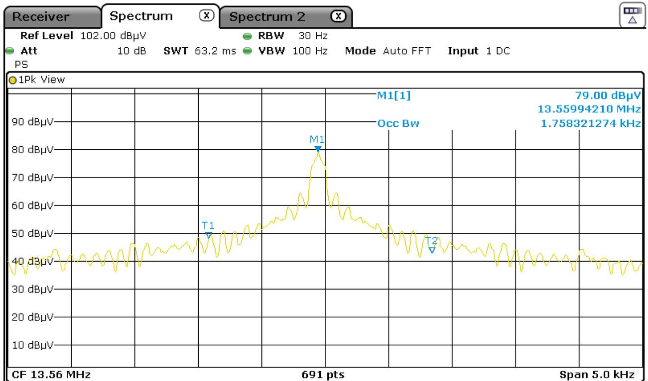
Figure 16: Chart of occupied bandwidth test, without tag, USB
