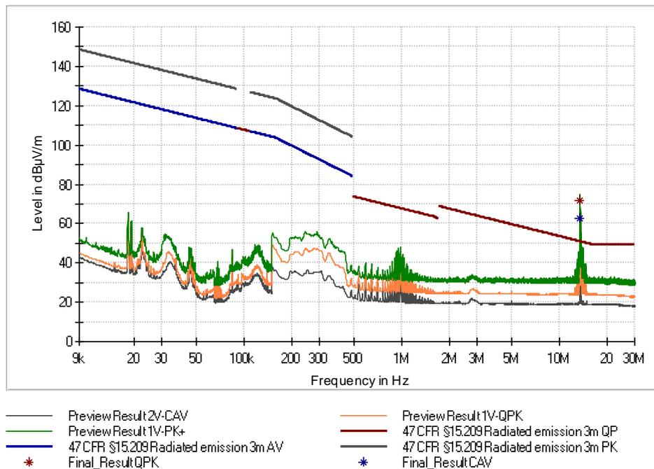
Figure 20: Chart of emissions test below 30 MHz, EUT position X, without tag, antenna in line at 3 m, USB
