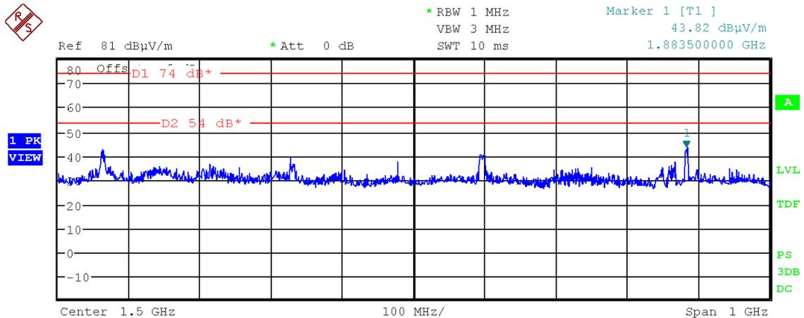
Figure 25: Chart of emissions test from 1 GHz to 2 GHz, EUT position X, with tag, antenna vertical, RS232
