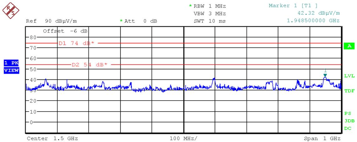
Figure 24: Chart of emissions test from 1 GHz to 2 GHz, EUT position X, with tag, antenna vertical, USB
