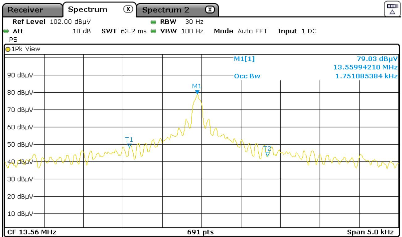
Figure 17: Chart of occupied bandwidth test, without tag, RS232
