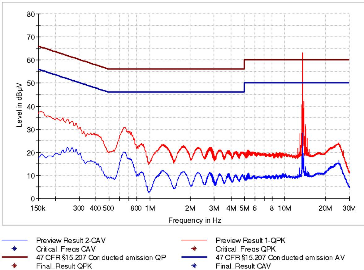
Figure 10: Chart of AC powerline conducted emissions on L1 – without termination, RS232
