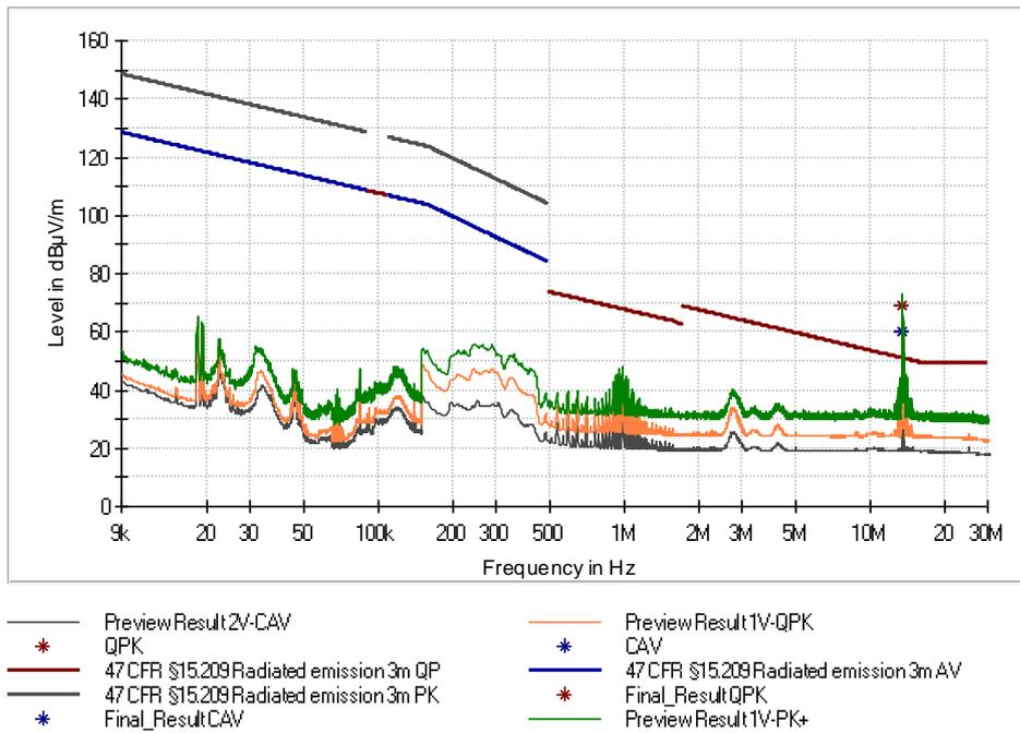
Figure 21: Chart of emissions test below 30 MHz, EUT position X, without tag, antenna in line at 3 m, RS232
