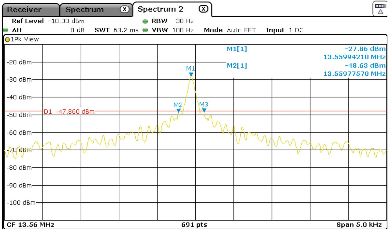
Figure 15: Chart of 20 dB bandwidth tests, with tag, RS232
