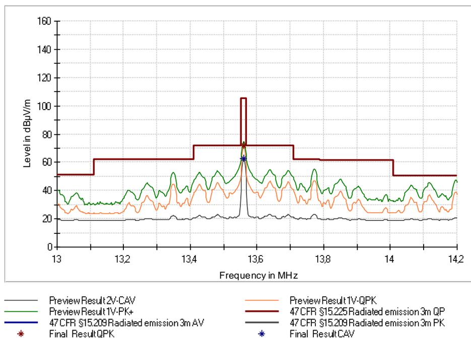
Figure 18: Chart of emission within the band 13.110 MHz to 14.010 MHz, EUT in position X, without tag, antenna in line at 3 m distance, USB
