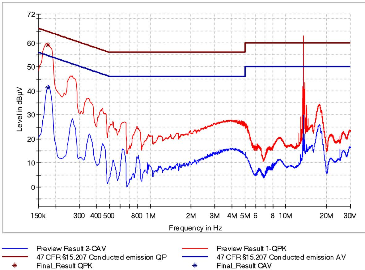
Figure 6: Chart of AC powerline conducted emissions on L1 – without termination, USB
