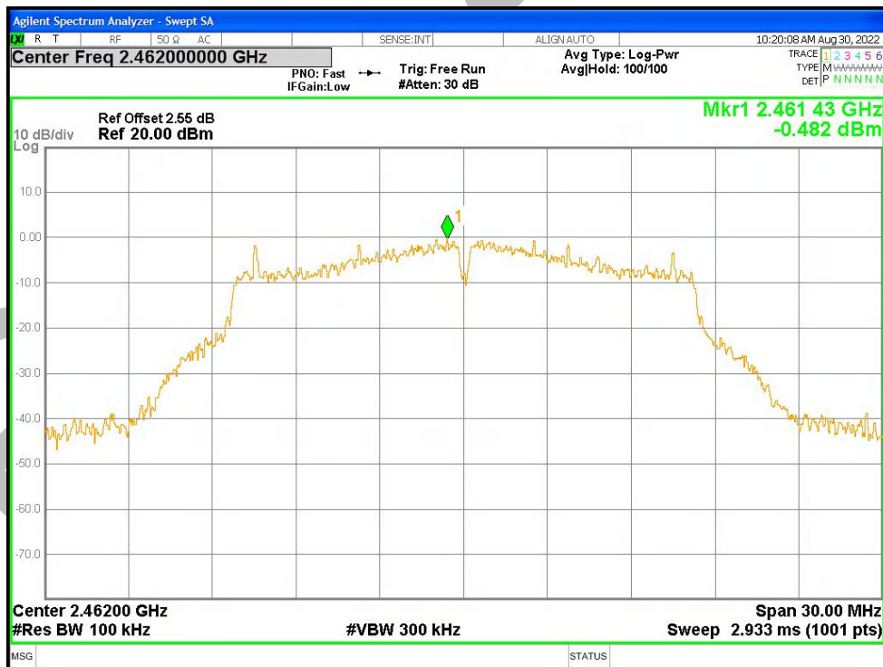
Tx. Spurious NVNT g 2462MHz Ant1 Emission
