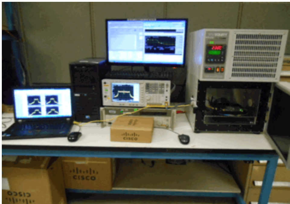
Title: Temperature / Frequency Stability Test Set Up
