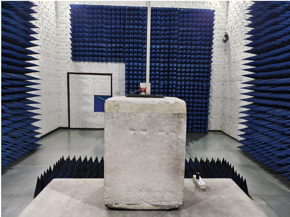
RADIATED EMISSION TEST SETUP ABOVE 1GHz
