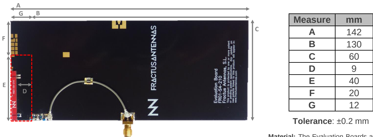
Figure 1 – EB_FR01-S4-210-M. Evaluation Board for providing operation in 2 frequency ranges, 698 – 960MHz and 1710 – 2690MHz.
